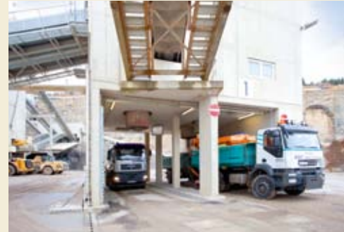
Parallel loadout: Simultaneous loadout at two points
