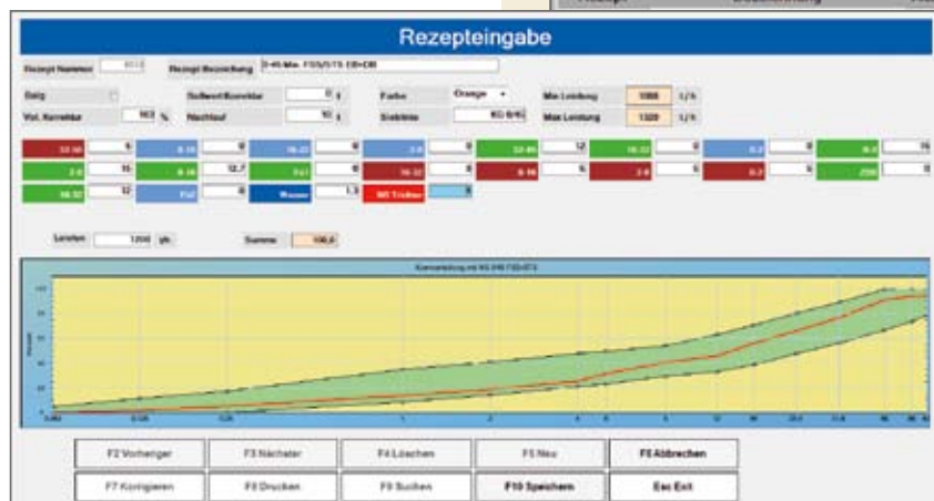
Recipe screen with lower and upper limits of particle-size distribution curve
