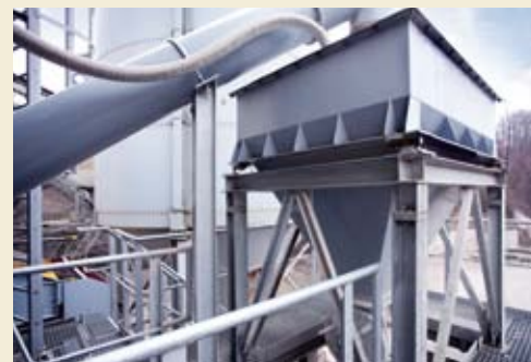
Hopper scale with screw feeder for gravimetric addition
